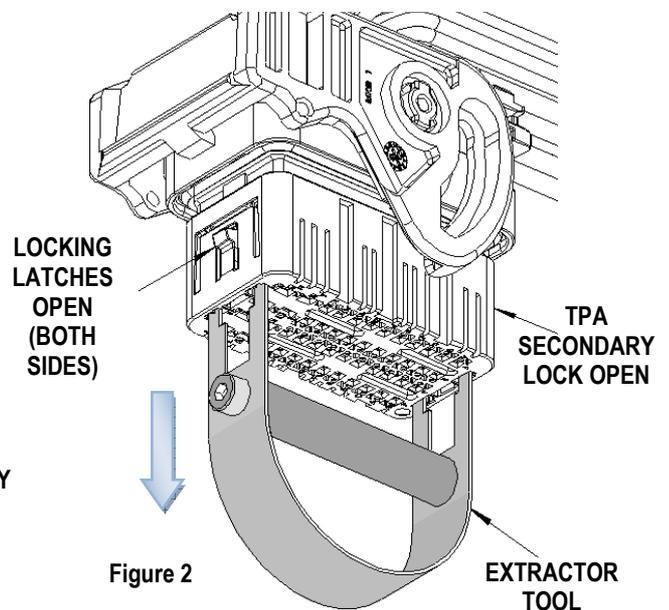
1. Insert the extractor tool into the (2) side slots of the (TPA) secondary lock on each sides until it stops. See Figure 1.
