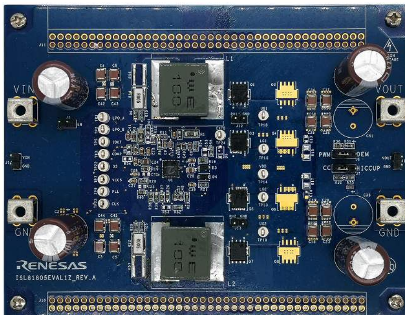
Figure 4. ISL81805EVAL1Z Evaluation Board, Top View
