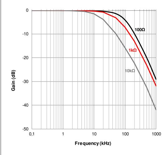
Testcondition: I<sub>C</sub>= 2mA; V<sub>CF</sub>= 2V; TA= 25°C
