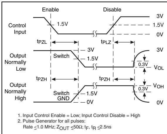
**Propagation Delay Diagram**
