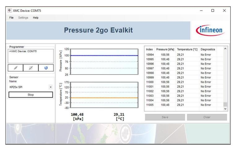
Real time graph for plotting pressure and temperature value.
