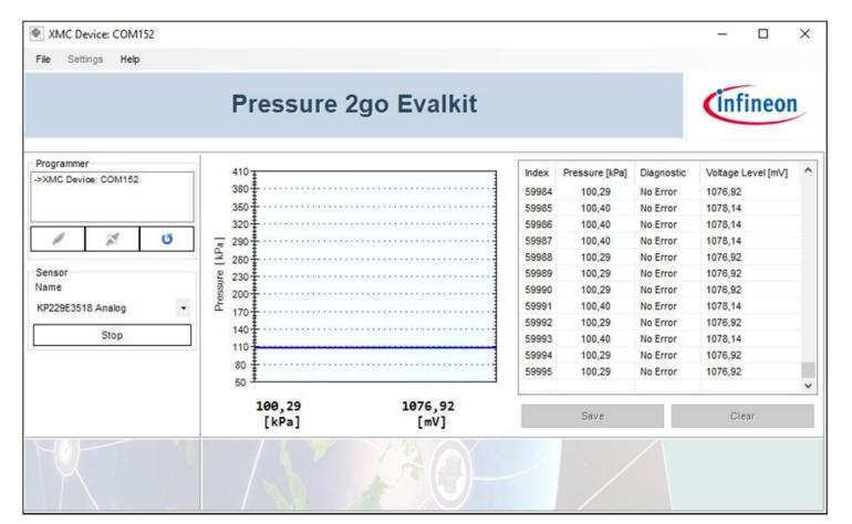
The sensor panel is configured for the corresponding sensor and you will see the specific controls. Real time graph for plotting the pressure value. Acquisition log to display all
