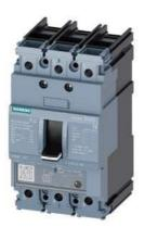
circuit breaker 3VA5 UL frame 125 breaking capacity class S 25kA @ 480 V 3-pole, line protection TM230, FTAM, In=100A overload protection Ir=100A fixed short-circuit protection Ii=5...10 x In cable connection on both sides
