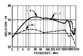
**Isolation vs. Frequency:** Level of  $f_L$  signal fed through to R- and I-port with respect to the level of the  $f_L$  signal at L-port. R-I Isolation plotted with  $f_L$  at 1500 MHz.
