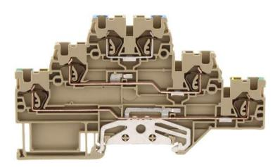
Three-level initiator terminal | Multi-wire terminal, Tension-spring connection, Mounting type: Mounting rail TS 35/7.5, Rated cross-section: 2.5 mm², Width: 5.1 mm, Colour: Beige
