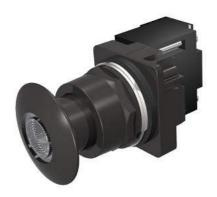
30mm BlackMax, Epoxy Coated Corrosion Resistant Complete Metal Unit Illuminated Push-Pull Operator Full Voltage, 12V AC/DC Incandescent Lamp Mushroom Head Cap Small 1 3/4" (44.5 mm) Metal, Black with Clear Lens 3 Position Momentary UL Listed, CSA Certified NEMA 1,3,3R,4,4X,12,13 & Automotive Standards
