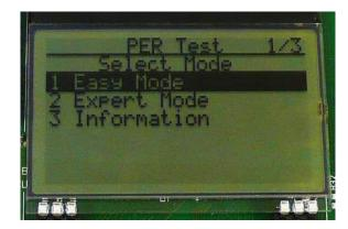
The PER test can be run is several modes. Easy Mode sets up a one-way test and uses default settings. This test is convenient for practical range testing.
