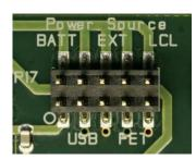
Depending on the power source, make sure you connect jumpers to the appropriate pins on the "Power Source" header. For instance, if you use batteries, use a jumper to short-circuit pin 1 and 2 on the header. See back side of board for explanation of the jumpers..
