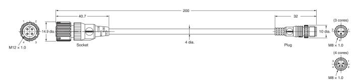
Note: For 3-core, M12 connectors, pin 2 is not connected internally.
