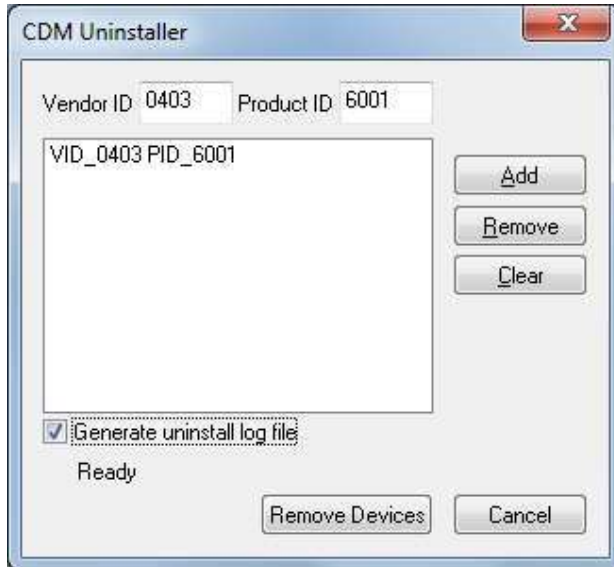
Figure 7: CDM Uninstaller after FTDI Vendor and Product ID have successfully been added
