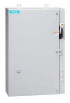
Non-reversing motor starter Size 4 Three phase full voltage Solid-state overload relay OLRelay amp range 50-200A 240V 50HZ / 277V 60HZ coil Combination type 150A circuit breaker Enclosure NEMA type 4/12 Water/dust tight for outdoors Standard width enclosure
