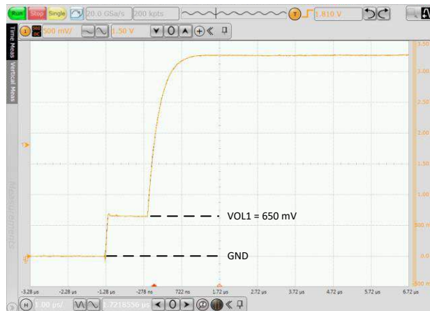
Figure 9-8. Side 1 ISO1640: Low-to-High Transition
