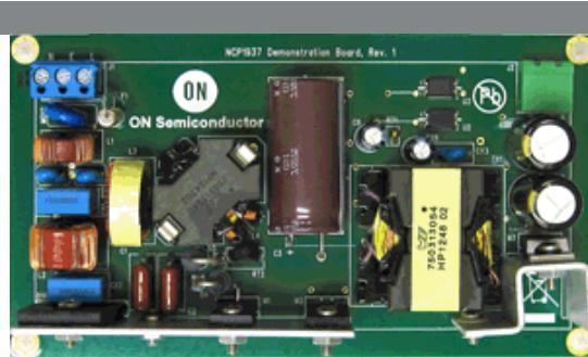
The quasi-resonant current-mode flyback stage features a proprietary valley-lockout circuitry, ensuring stable valley switching. This system works down to the 4th valley and toggles to a frequency foldback mode with a minimum frequency clamp beyond the 4th valley to eliminate audible noise. Skip mode operation allows excellent efficiency in light load conditions while consuming very low standby power consumption.
