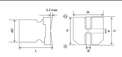
Unit: mm Size L +0.1 -0.4  $P^{*2}$ W±0.2 C±0.2 øD±0.5 H±0.2 R code 5.0 5.9 5.3 5.3 6.0 0.6 to 0.8 1.4 B6 C6 6.3 5.9 6.6 6.6 7.3 0.6 to 0.8 2.1 8.0 6.9 8.3 8.3 9.0 0.6 to 0.8 E7 3.2 E12 8.0 11.9 8.3 8.3 9.0 0.8 to 1.1 3.2 F10 10.0 10.0<sup>\*1</sup> 10.3 10.3 11.0 0.8 to 1.1 4.6 10.0 F12 12.6 10.3 10.3 11.0 0.8 to 1.1 4.6
