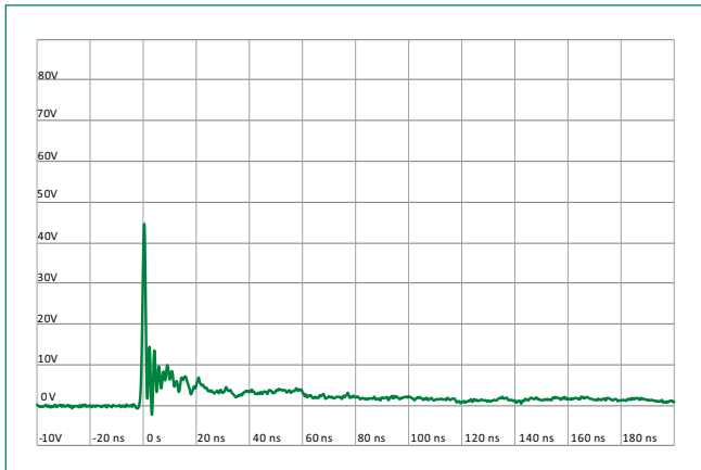
IEC 61000-4-2 +8 kV Contact ESD Clamping Voltage
