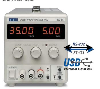
A simple command set allows remote control of voltage, current and output enable together with read-back of metering values and operational status. Local control is via three rotary encoders providing rapid and accurate setting of voltage and current during bench use. The EX355P-USB has similar functionality but is controlled via a USB
