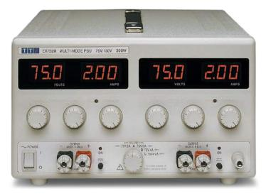
As a dual, each output provides 0 to 75V at 0 to 2A (mode A). As a single, the output can be selected as either 0 to 75V at 0 to 4A (mode B) or 0 to 150V at 0 to 2A (mode C). In single modes, the unused half of the unit becomes completely inoperative and its displays are blanked.
