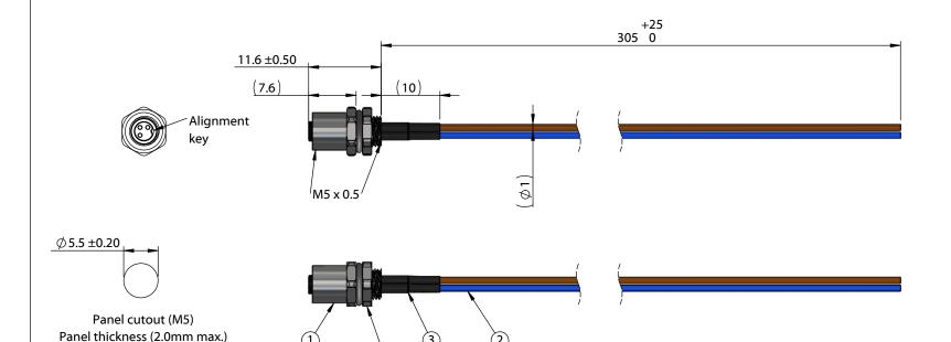
Install from outside of the panel, attach nut and tighten from within.
