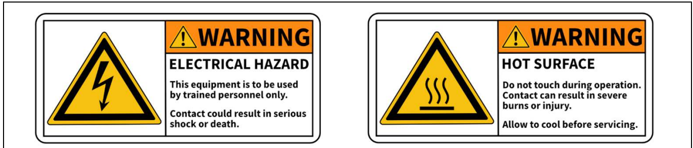
Figure 2 Electrical hazard and hot surface warning
