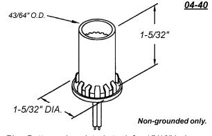
Plug Button: zinc plated steel, for 15/16" hole for panel thickness range 1/32" to 5/64".
