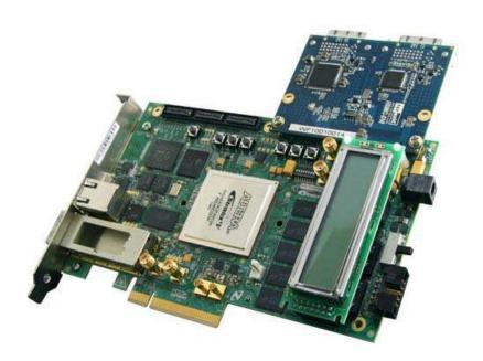
The Stratix V GX FPGA Video Development System fills the need for the highest bandwidth, best performance video applications. The kit features an extensive feature-set of memories, including DDR3, QDRII+, and RLDRAM II. The QSFP optical cage, PCIe x8 edge connectors, SDI, and gigabit Ethernet options allow for blazingly fast interfacing with peripherals.
