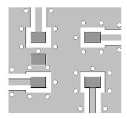
Recommended PCB layout shown above uses 1.6 mm FR4, rounded coplanar wave guide, transmission line width 0.70 mm and gap 0.57 mm.
