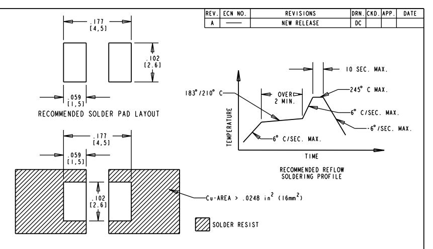
PAD LAYOUT FOR IMPROVED HEAT DISSIPATION
