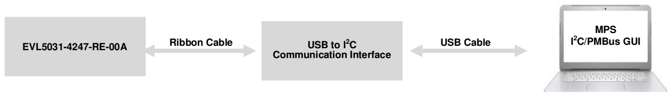
Figure 1: EVKT-MP5031 Evaluation Kit Set-Up
