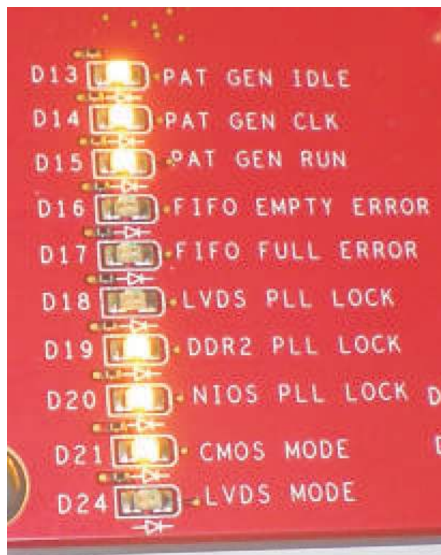
Figure 16. TSW3100 LED Status With Test Pattern Running
