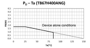
This value is dependent on a substrate pattern and mounting conditions. Moreover, when ambient temperature is high, permissible power consumption becomes small.
