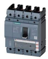
circuit breaker 3VA5 UL frame 250 breaking capacity class M 35kA @ 480 V 4-pole, line protection TM230, FTAM, In=200A overload protection Ir=200A fixed short-circuit protection Ii=5...10 x In N conductor unprotected without connection
