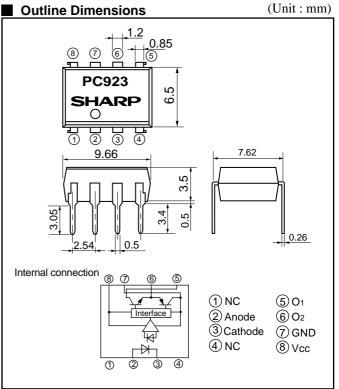
\* "OPIC" (Optical IC) is a trademark of the SHARP Corporation. An OPIC consists of a light-detecting element and signalprocessing circuit integrated onto a single chip.
