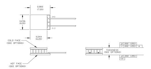
Solder Construction: 138°C, Bismuth Tin Tlam Substrates
