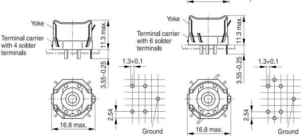
\*) This recess must be on the side of the grounding pin to ensure that the yoke locks in position.
