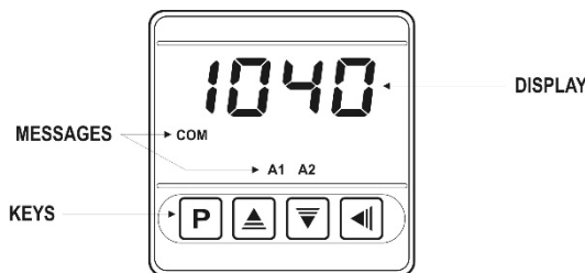
Figure 06 - Identification of the front panel parts
