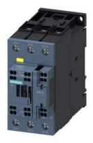
power contactor, AC-3e/AC-3, 65 A, 30 kW / 400 V, 3-pole, 175-280 V AC/DC, 50/60 Hz, with integrated varistor, auxiliary contacts: 1 NC, main circuit: screw terminal, control and auxiliary circuit: spring-loaded terminal, size: S2, F-PLC-IN
