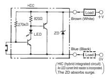
Note: The load may be connected to either the +V or 0 V terminal.
