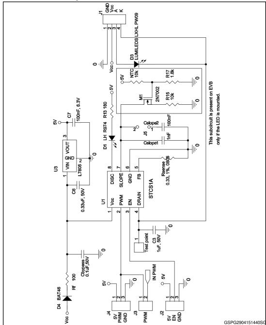
Figure 1: STEVAL-ILL014V1 circuit schematic
