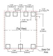
\* Do not route any traces in the keep out area. It is recommended the next layer under the keep out area is to be ground plane.
