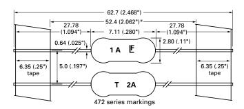
Coating Diameter (max): 0.5A-3.0A: 2.80mm 5.0A: 2.90mm
