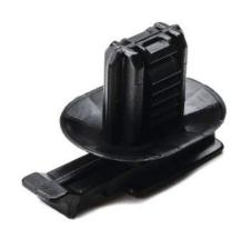
HellermannTyton Connector Clips provide a single method to mount connectors to various surfaces in a variety of applications. Highly engineered designs feature anti-rattle discs, anti-rotation oval fir trees and clamps for mounting on edges.
