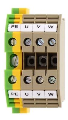
Four-wire motor-connection block, Screw connection, Mounting type:Mounting rail TS 35/7.5 and TS 32, Rated cross-section: 4 mm², Colour: Multi-coloured
