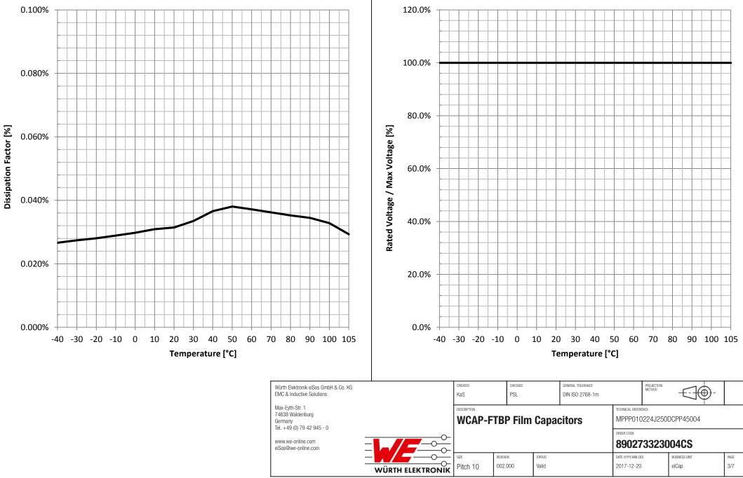
**Rated Voltage vs. Temperature:**
