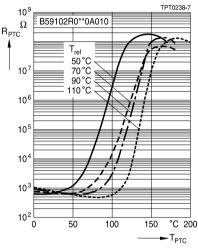
PTC resistance  $R_{\text{PTC}}$  versus PTC temperature  $T_{\text{PTC}}$  (measured at low signal voltage)
