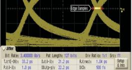
Figure 8. Main Link Input With 10-Inch Trace; TMDS Sink
