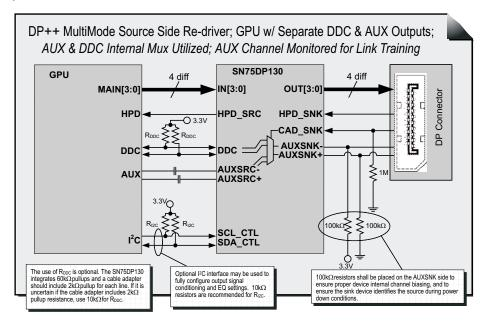
Figure 21. DP++ Dual-Mode in a Split AUX/DDC Configuration
