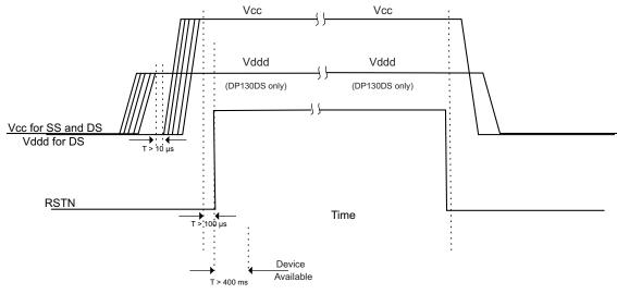
Figure 34. Power-Up and Power-Down Sequence
