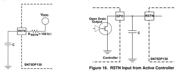
Figure 15. External Capacitor Controlled RSTN
