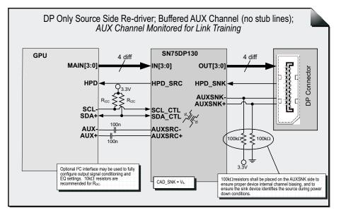
Figure 22. DP Only Configuration with AUX Pass Through
