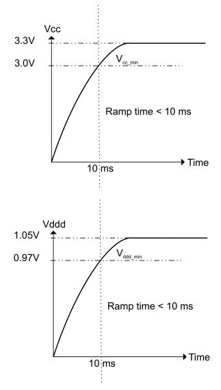
Figure 35. V<sub>CC</sub>/V<sub>DDD</sub> Ramp Recommendation
