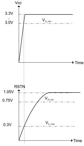
Figure 36. RSTN Voltage Thresholds
