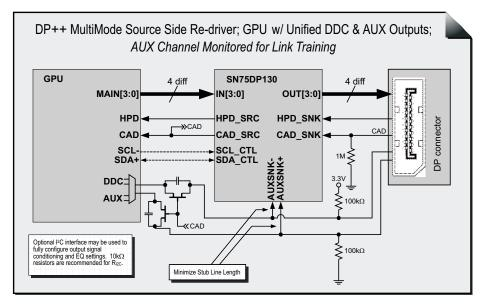
Figure 23. DP++ Dual-Mode Configuration with AUX Monitor
