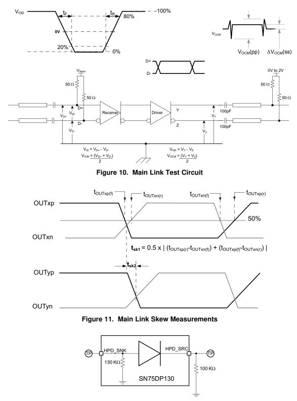
Figure 12. HPD Test Circuit
