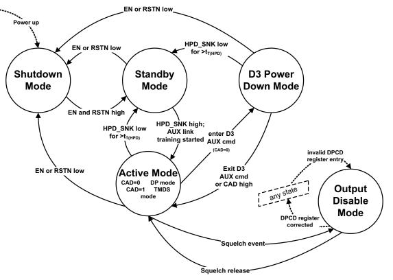
Figure 18. SN75DP130 Operating Modes Flow Diagram
