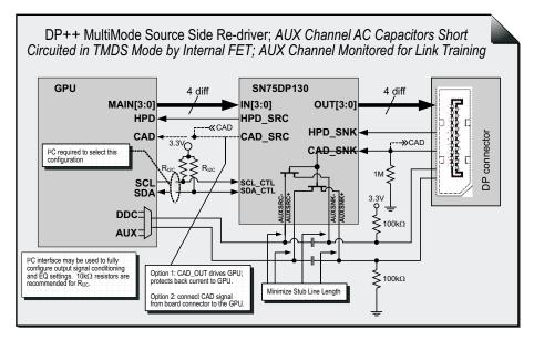
Figure 24. Alternate Low-BOM DP++ Dual-Mode Configuration
