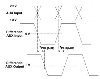
Figure 14. AUX Delay Measurement
