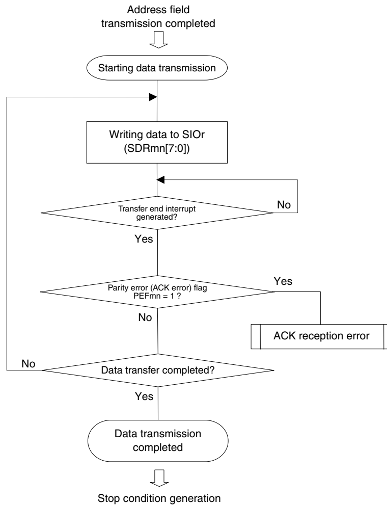
Figure 14-104. Flowchart of Data Transmission
