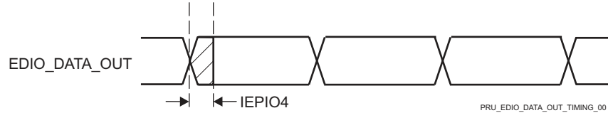
Figure 7-100. PRU_ICSSG IEP Digital IOs Timing Requirements
