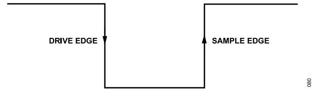
Figure 78. SPI Mode 0 SCLK Edges
