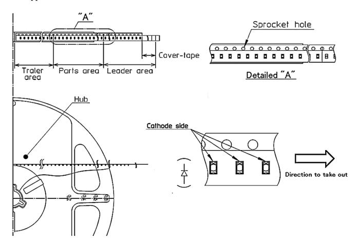
Note "-TR" means cathode side of LEDs should be placed on the sprocket-hole side.
