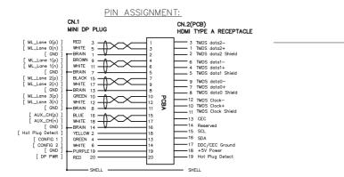
Electrical performance test: (MINI DP TO HDMI machine testing) 1. signal source UXGA: 1280\*720P, 1920\*1080P
