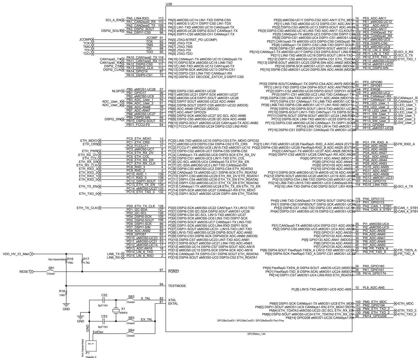
Figure 12. AEK-MCU-C4MLIT1 schematic - MCU I/O signals
