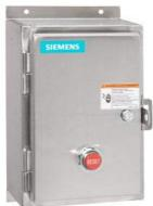
Non-reversing motor starter Size 1 Three phase full voltage Solid-state overload relay OLRelay amp range 5.5-22A 550/575-600 50/60HZ coil Combination type Water/dust tight non-corrosive
