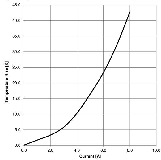
CHECKED REVISION DATE (YYYY-MM-DD) GENERAL TOLERANCE CSo 001.003 2019-05-06 DIN ISO 2768-1m **WE-WPCC Wireless Power** Würth Elektronik eiSos GmbH & Co. KG **Transfer Transmitter Coil** ORDER CODE EMC & Inductive Solutions Max-Eyth-Str. 1 760308101304 74638 Waldenburg SIZE/TYPE STATUS Tel. +49 (0) 79 42 945 - 0 BUSINESS UNIT PAGE www.we-online.com 3/6 Ø 48 eiSos Valid eiSos@we-online.com
